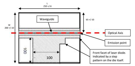
Figure 1: Drawing of 250  $\mu$ m x 200  $\mu$ m laser diode chip with emission point and optical axis
