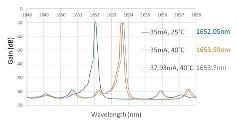
Figure 3: Precise tuning of wavelength to 1653.7 nm via TEC and current tuning
