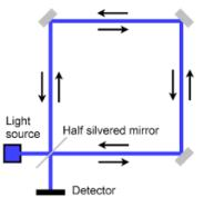
If the apparatus rotates clockwise, the beam moving clockwise effectively travels a slightly longer path than the beam travelling counterclockwise (and vice versa) creating a path difference between the two beams of light. As shown below, the red and blue dots represent counter-propagating photons, the grey dots represent molecules in the loop material.
