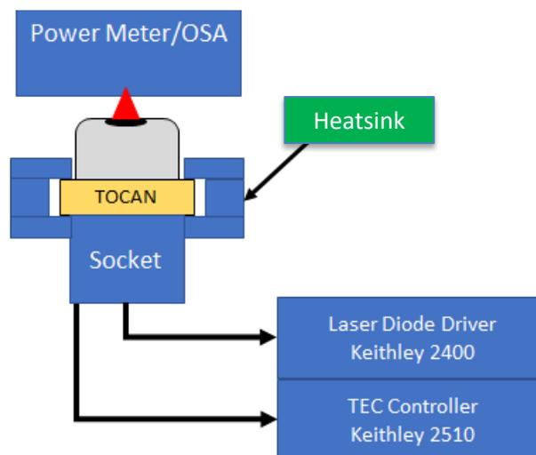
Figure 2: Illustrative testing set-up for 1653nm DFB device packaged in TO-can
