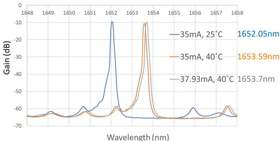
Figure 3: Precise tuning of wavelength to 1653.7 nm via TEC and current tuning
