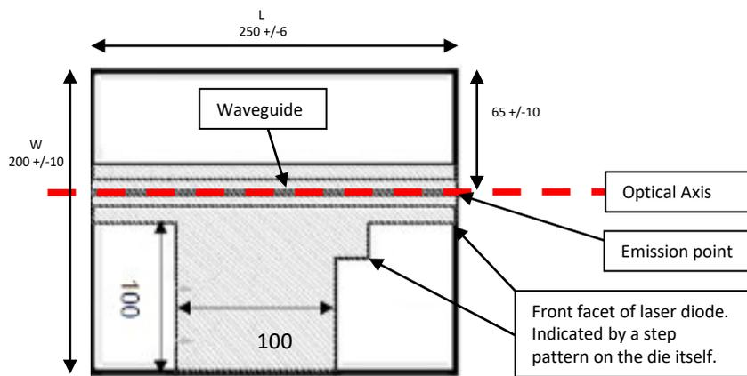
Figure 1: Drawing of 250  $\mu\text{m}$  x 200  $\mu\text{m}$  laser diode chip with emission point and optical axis
